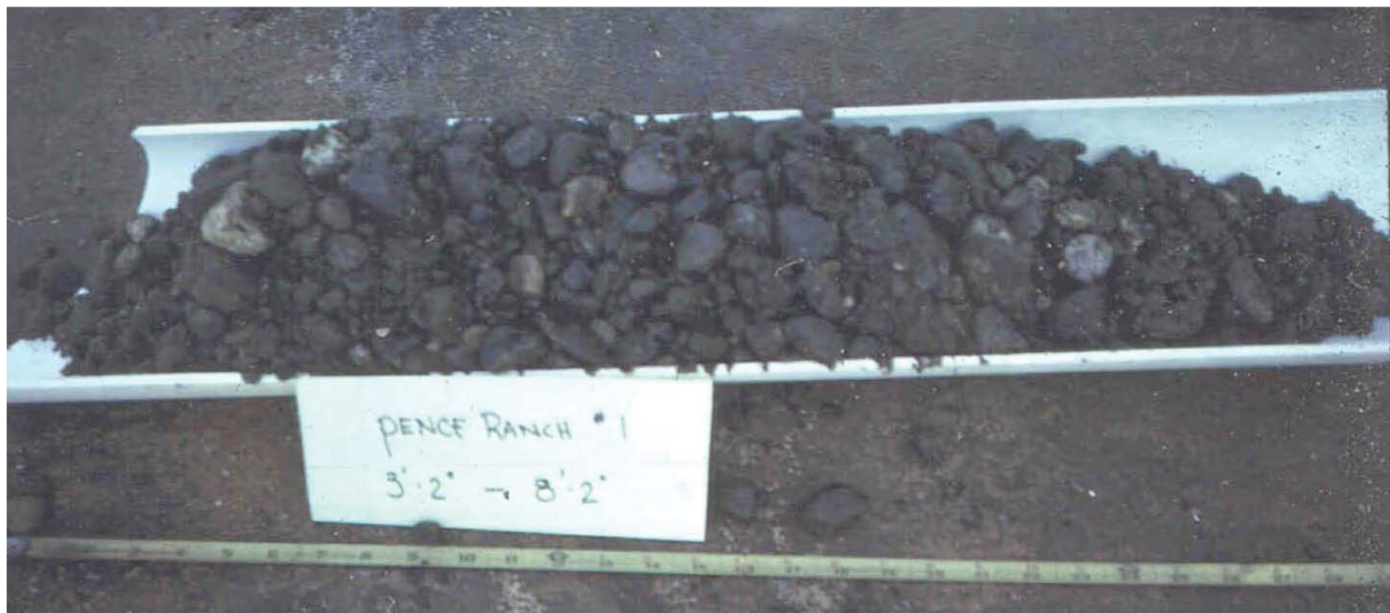
Gravel Sample Taken from Layer that Liquefied beneath Pence Ranch
