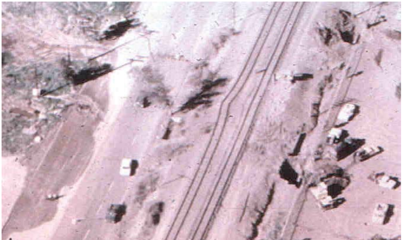
Craters and Flooding Due to Pipeline Breaks, San Fernando Juvenile Hall Lateral Spread
