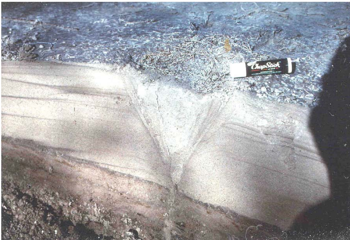
Cross section of sand boil generated by 1981 Westmorland, Calif. earthquake
